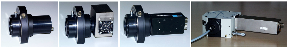
Fig. 53: Detectors of the bh non-descanned FLIM systems. Left to right: R3809U MCP PMT, PMC-100, H7422P-40, bh MW-FLIM detector
